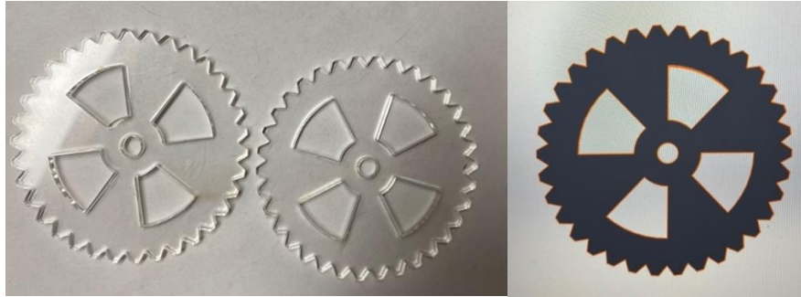
Figure 17 The first laser cut flywheel prototypes and SolidWorks design.
