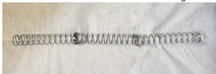
Figure 22 Connected springs for reloading mechanism.
