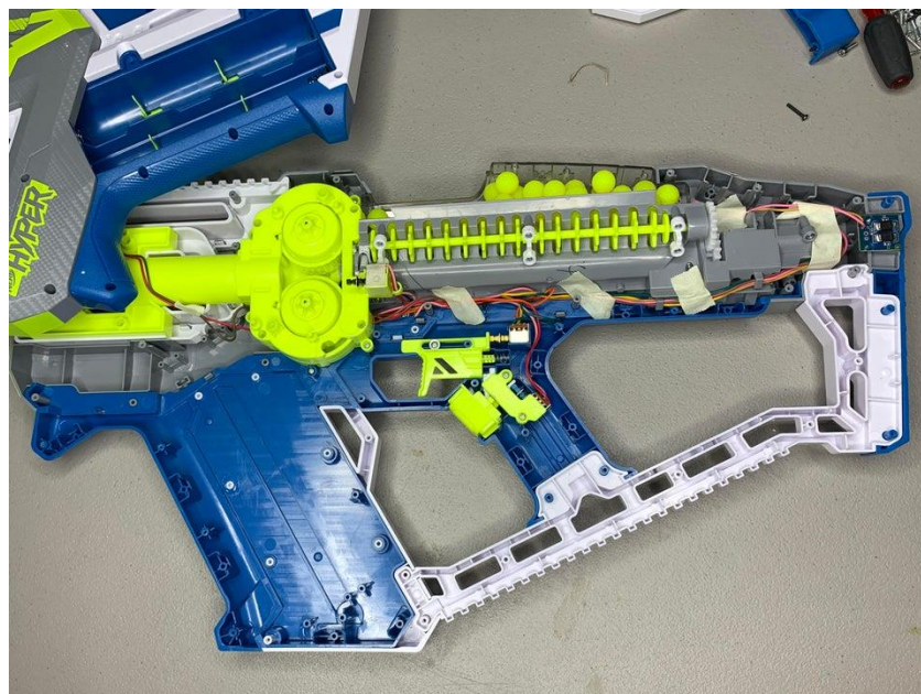
Figure 3 The Hyper Nerf® Gun launching system [2].
