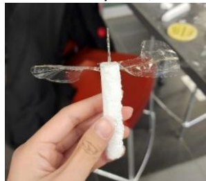
Figure 10 Incorporating a leading-edge shaped wing.
