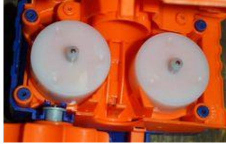
Figure 15 Nerf® gun's inner flywheel mechanism [8].
