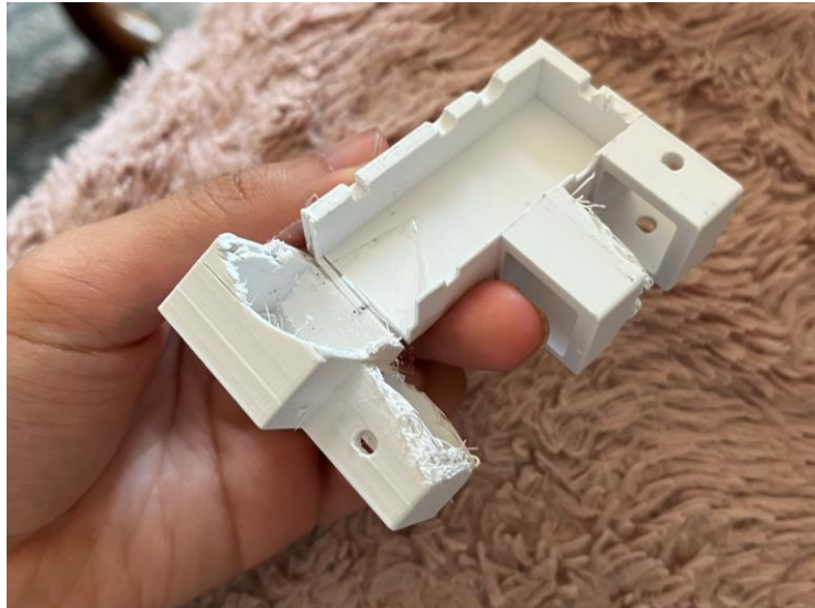
Figure 14 The third prototype snapped while the TT motor was seated
